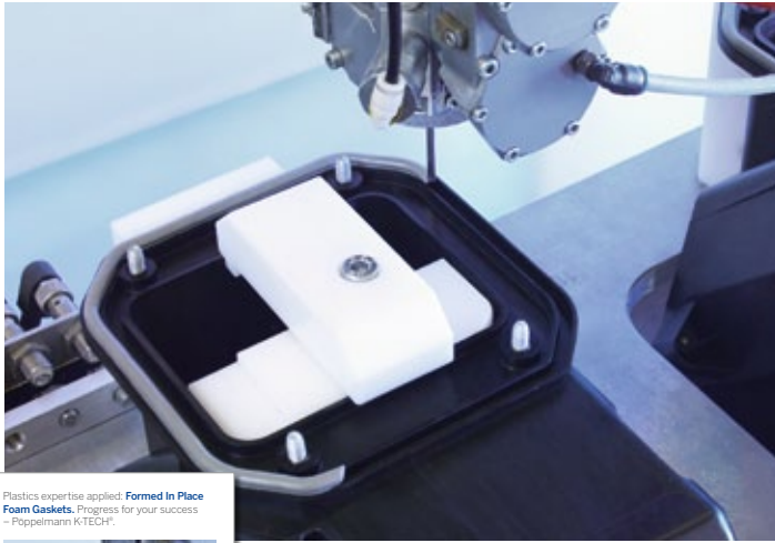
Cover for control unit boxes with a PUR gasket applied directly into the component
