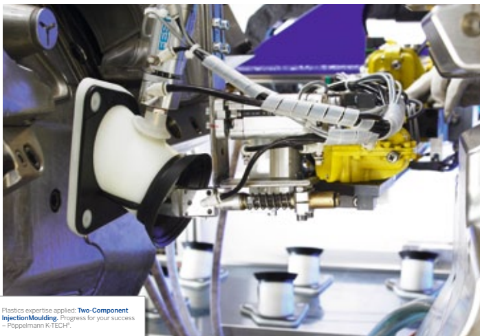
Effective moisture protection: 2C floor sockets for attaching side member panelling in cars
