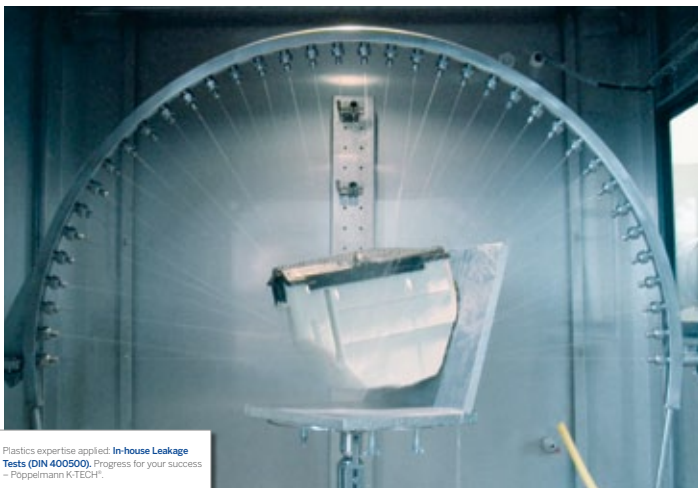
2C sleeves fitted precisely to the overall leak tightness requirements of the respective control unit boxes
